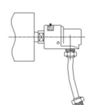
2. After assembling the hoses, install the joint to the machine. When installing, pay attention not to install eccentrically.
