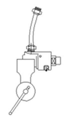
1. First hold the rear of the joint in a bench vise and assemble the flexible hoses.
