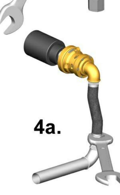
4.Connect supply and return lines to the hoses. Control the flexibility of the hoses. Be sure that the hoses are flexible and will be flexible under the pressure and temperature of the medium. Never install the joint directly to the supply and return pipes.
