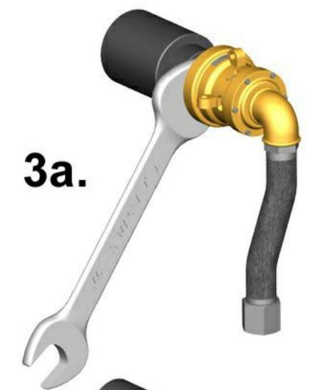
3. After assembling the hoses, install the joint to the machine. When installing, pay attention not to install eccentrically.
