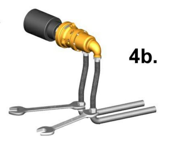
5. After assembling, check if running is smooth. If not, disassemble the joint from the machine and assemble it again.
