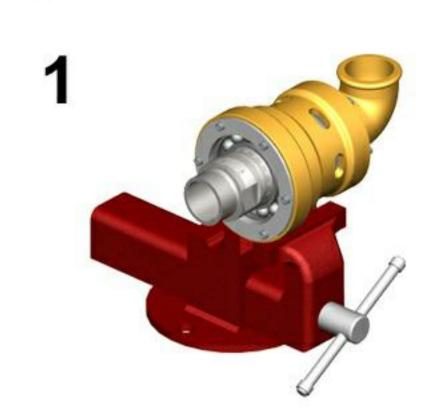
1. First hold the rear of the joint in a bench vise.
